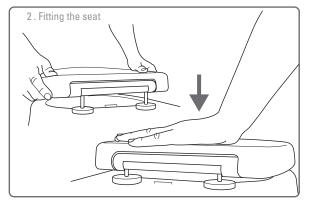
Align and insert the pins into the seat hinge sockets and firmly press down until you hear them 'click' into position.
