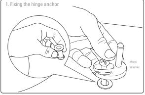
Place the Top Fix Inserts into the fixing holes in the toilet pan. Insert the screws within the Hinge Anchors and washers inserted as shown and begin to tighten the screws until they are loosely secured, to allow for adjustment of the seat on the pan.
