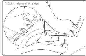
This toilet seat is designed for quick and easy removal when cleaning the toilet pan. To activate the quick release lift the lid and seat up. Pinch the button in the centre of the hinge bar inwards and lift. To replace the seat align the sockets with the pins and firmly press down until you hear them 'click' into position.
