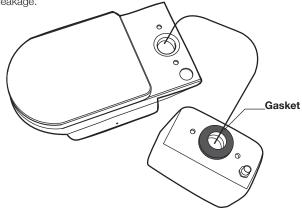
Insert the cistern fitting bolts arranging the components as shown in the diagram below.
