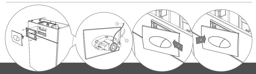
Cut aperture 172 mm x 105mm. Check for obstructions before cutting. Screw mounting bracket to the unit
