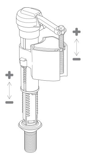
By adjusting the fill valve the water level can either be increased or decreased accordingly
