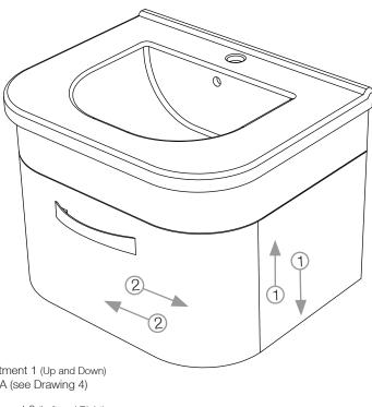
To make adjustment 1 (Up and Down) turn screw A (see Drawing 4)
