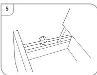
To make adjustment 1 (Up and Down) turn screw A (see Drawing 4)
