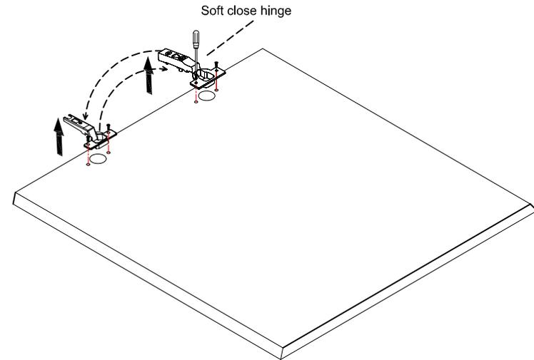
**3: Exchange the two hinges and attach them to the door.**
