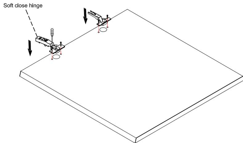
**4: Reattach the door to the carcass, and insert the plug.**
