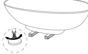
Make sure the four feet underneath the plinth level with the bottom of the plinth. The feet are for leveling only and not to bear the weight of the bath. Please adjust any of the feet as the above diagram if the floor is not perfect flat.
