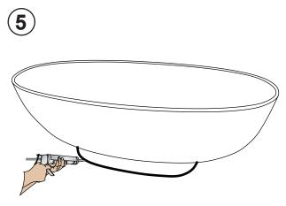
Securing your bath to the floor: When the bath is in position and the installation is complete, it is recommended that you apply a bead of silicone around the bottom of the plinth to secure it to the floor.
