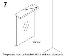
The product must be installed with a minimum distance of 150mm between the infrared sensor and an adjacent countertop or obstruction to ensure correct function of the sensor.
