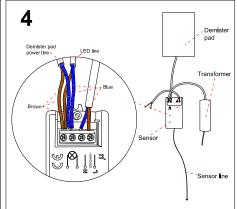
Please follow this step to connect the demister pad if any. Remove the back cover of the sensor and connect cables according to above diagram. Then put the cover back on.
