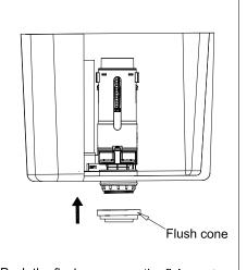
Push the flush cone over the fixing nut, ensure that it is flat, and there will be no leakage between cistern and pan.
