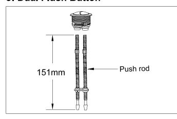
Screw the push rods out of the button, and cut the push rods to a length of 151mm as shown in the diagram on the left hand side.
