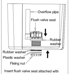
rubber washer into cistern flush hole. Then install the rubber washer, plastic washer, and tighten with the fixing nut.
